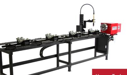
torch in the manual mounting with throw lever and cam lock clamps, including an easy manual adjustment for torch bevel to decrease hand grinding and weld preperation finish work. These features all reduce the time between cutting operations and lead to real efficiency improvements.
