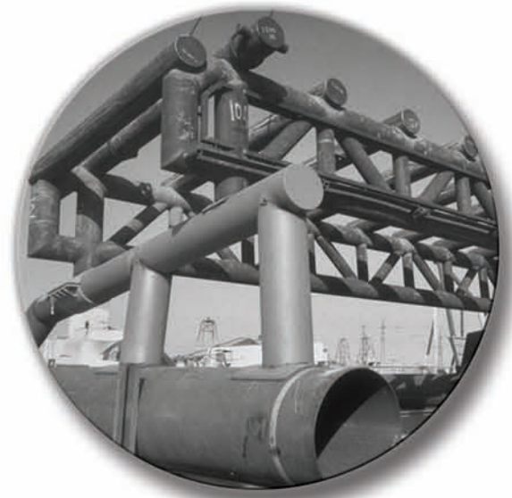
Structural support piping requires proper fit-up of brace members. Weld preparation angles made to stringent AWS specifications enhance structural integrity and reduce grinding and filling labor.
